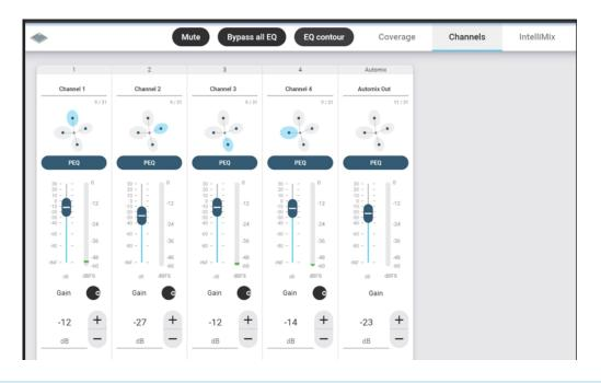
Go to the Automix page. Use the faders to adjust a channel's gain before it reaches the auto-mixer and therefore affects the automixer's gating decision.
